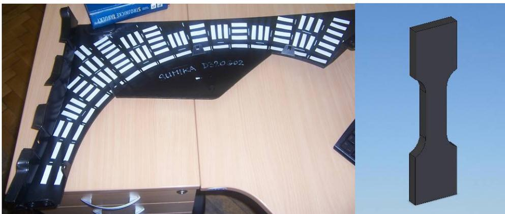
**Fig. 1.** Lay-out of specimens cut out from a plastic car bumper
