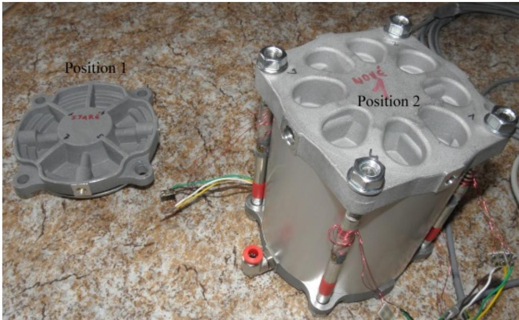
**Fig. 6.** Schematic connection of the lid's variants (on the left is old lid and new lid is on the right)
