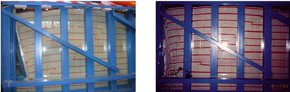
**Fig. 2.** Views at left lateral sides of the samples (the moved front wall is left) at the ends of the experiments with passive pressure during rotation about the top: a) (left) Experiment E3/0,2 with maximal movement of the toe of 158.8 mm. b) (right) Experiment E5/0,2 with maximal movement of the toe of 226.9 mm.
