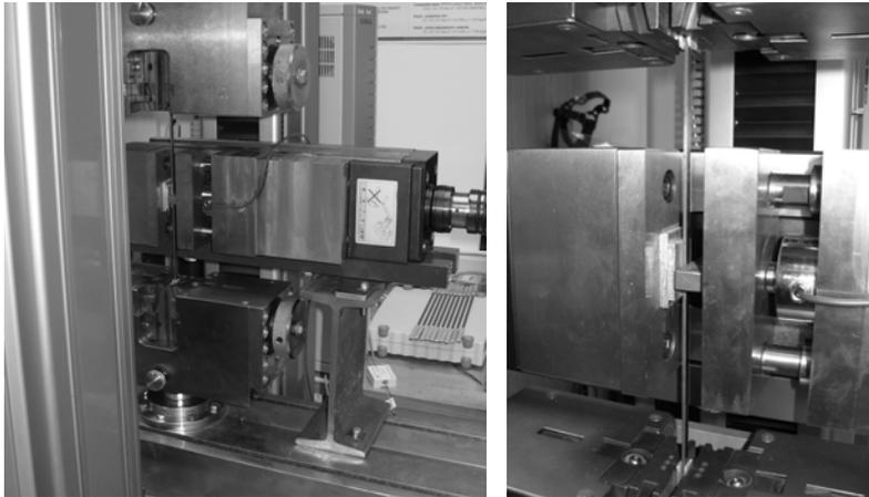
Fig. 2. Testing machine with additional compression device
