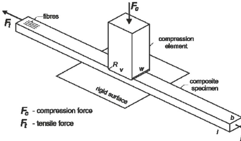
Fig. 1. Schema of biaxial test
