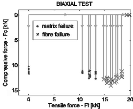
**Fig. 5.** Dependence of specimen strength on the combination of tensile and compression forces
