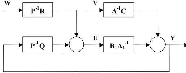
Fig. 2. Block diagram of the 2DOF control system
