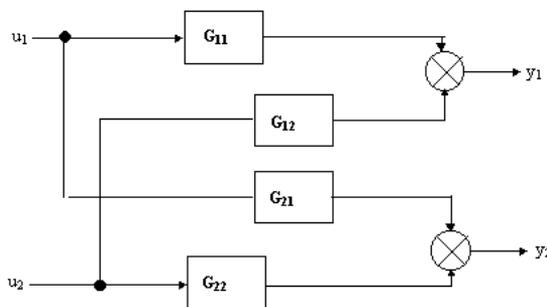
Fig. 1. A two input – output system - the “P” structure
