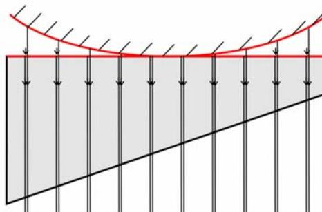
**Fig. 1.** Principle of Fizeau interferometry
