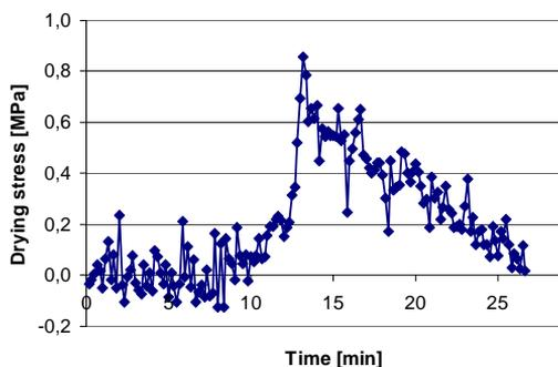
**Fig. 4.** Drying stress evolution during drying of a particular slurry sample
