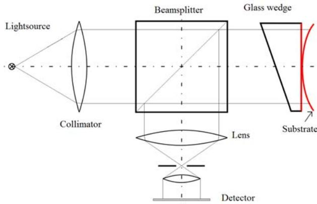
**Fig. 2.** Experimental setup of Fizeau interferometer
