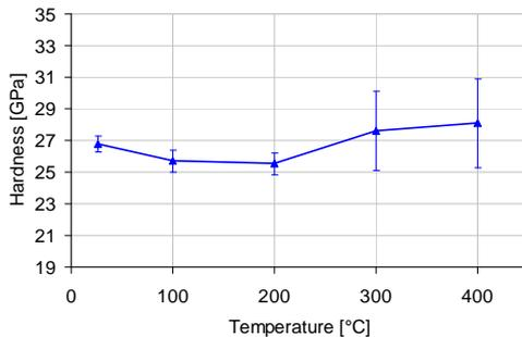
**Fig. 6.** Hardness of a-B<sub>4</sub>C films measured at different temperatures in air.
