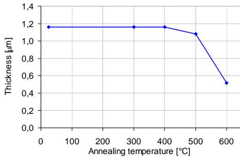
**Fig. 2.** Thickness of a- $B_4C$  films as a function of annealing temperature in air
