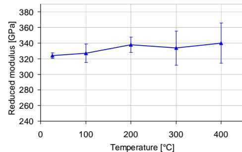
**Fig. 7.** Reduced elastic modulus of a-B<sub>4</sub>C films measured at different temperatures in air.
