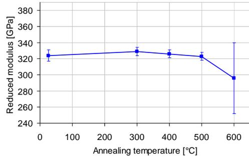
**Fig. 5.** Reduced elastic modulus of a-B<sub>4</sub>C films as a function of annealing temperature in air.
