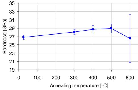
**Fig. 4.** Hardness of a-B<sub>4</sub>C films as a function of annealing temperature in air.
