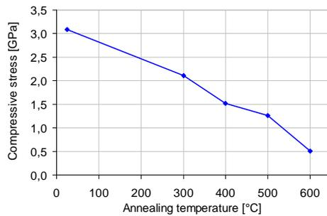
**Fig. 3.** Compressive stress of a- $B_4C$  films as a function of annealing temperature in air
