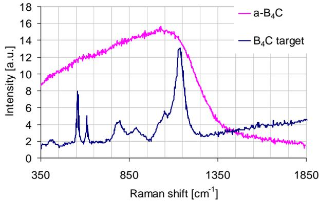
**Fig. 1.** Raman spectra of studied amorphous boron carbide thin film and polycrystalline  $B_4C$  target
