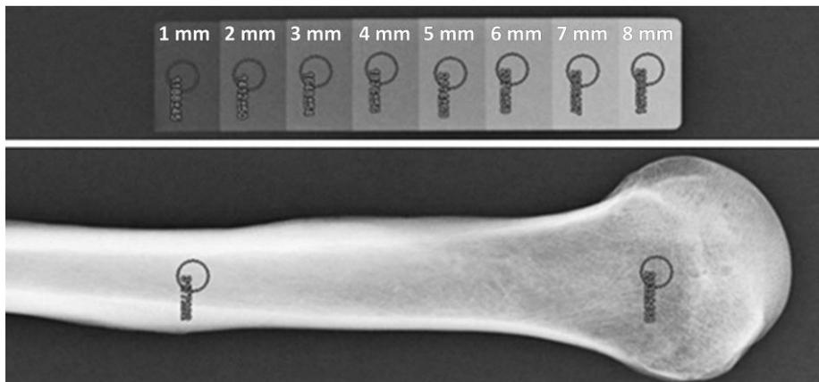
**Fig. 1.** An example of the optical densities of the X-ray film measurements
