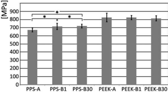
Fig. 2. The ultimate strength in bending (\* denotes statistically significant differences, Newman-Keuls post-hoc test,  $\alpha = 0.05$ )
