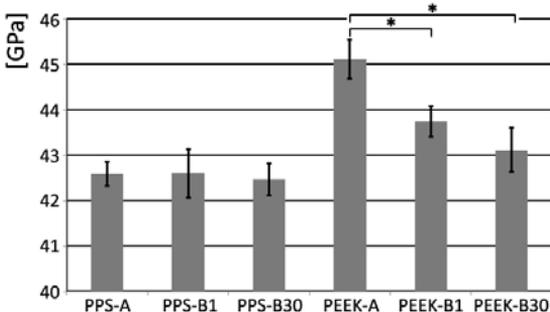
Fig. 3. The modulus of elasticity in bending (\* denotes statistically significant differences, Mann-Whitney post-hoc test,  $\alpha = 0.05$ )
