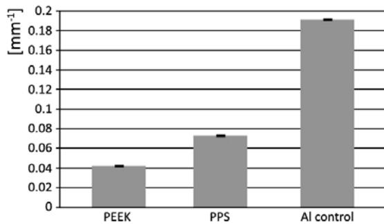
**Fig. 6.** Linear absorption (all values display statistically significant differences, Mann-Whitney post-hoc test,  $\alpha = 0.05$ )
