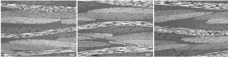
**Fig. 5.** Micrographs of polished sections of T300/PEEK composites (from left: A, B1, B30)
