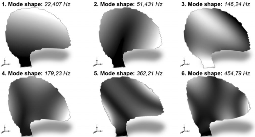
**Fig. 6.** The first six eigen frequencies and eigen shapes of the blade
