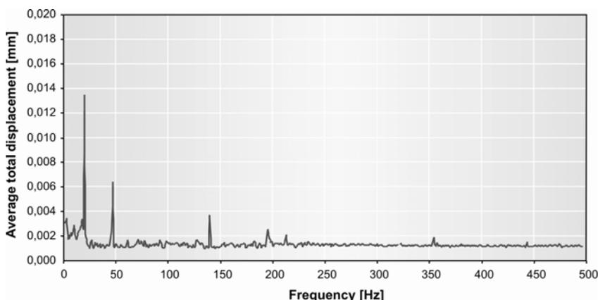
**Fig. 8.** The average frequency spectrum of absolute displacements of the blade measured by Q-450
