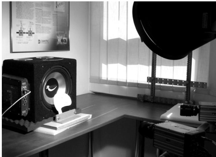
**Fig. 7.** A measuring of eigen frequencies of the fan blade by Q-450 system
