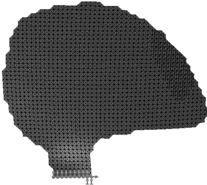
**Fig. 5.** Meshed model of the fan blade
