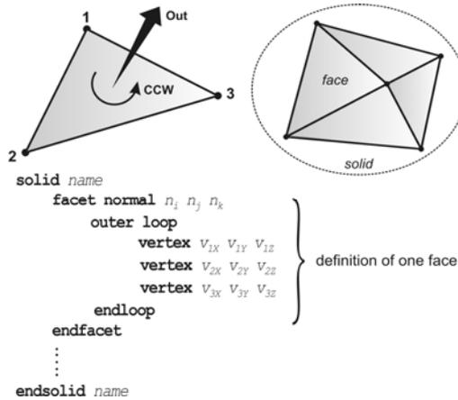
Fig. 2. Syntax for an ASCII STL file
