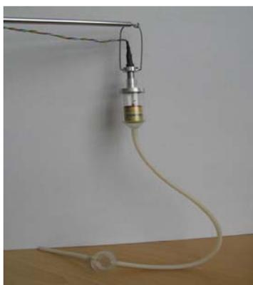
**Fig. 2.** Tube of laboratory device with the float and measuring sensor
