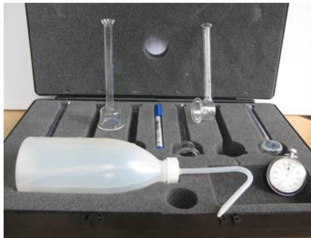
**Fig. 1.** Set of glass Karsten tubes for measurements on vertical and horizontal surfaces with a bottle of water for filling the tubes and stop-watch for time measurement.
