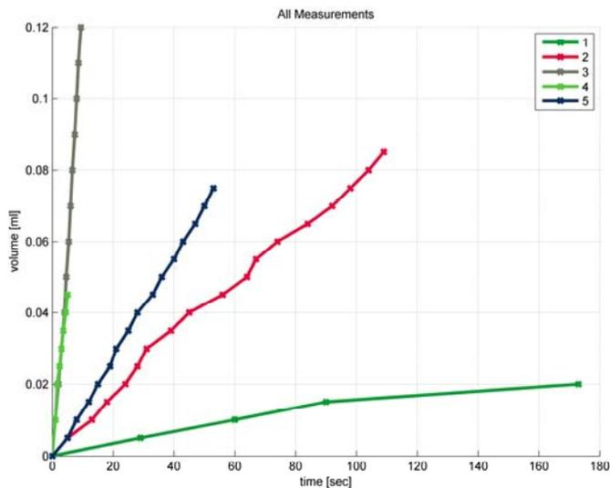
**Fig. 5.** Evaluated data from in situ measurements on differently deteriorated opuka stone – from a rather compact (1), through slightly degraded (2) to seriously deteriorated and cracked (3) and (4). Line (5) relates to a vertically cracked part of the relatively compact stone on which the (1) measurement was done.
