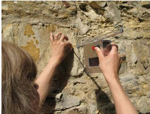
**Fig. 4.** Recording water absorption into opuka wall using “electronic” stop-watch and capillary tube with flexible outlet arrangement and cigarette filter contact medium.
