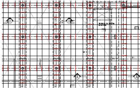
**Fig. 1.** Snapshot of the General Arrangement of Level 2 beams, slabs and scaffolding layout.
