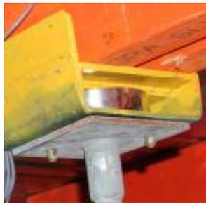
**Fig. 4.** Load cell contained in U-head support.
