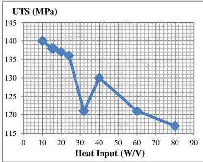
**Fig. 4.** Interacting Effect of V and W on Ultra Tensile Strength of the as welded A356-SiC composites
