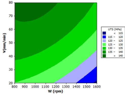
**Fig. 5.** The UTS contour result of RSM
