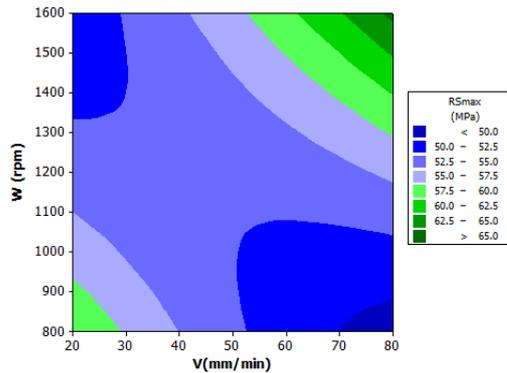
**Fig. 8.** The maximum of residual stresses contour result of RSM
