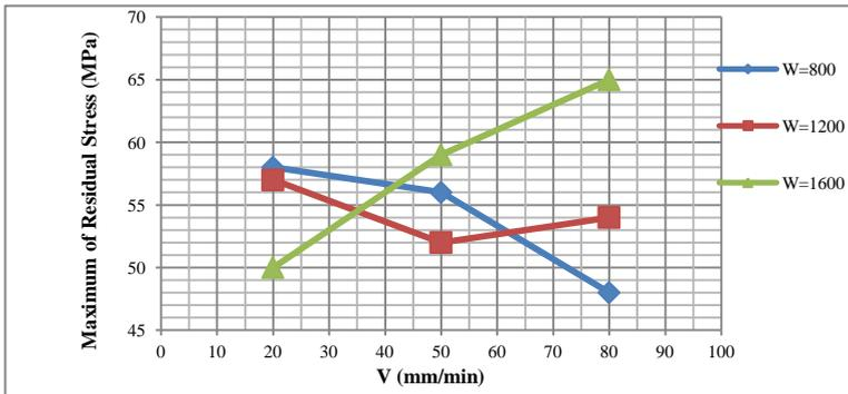
**Fig. 6.** Effect of V (transverse speed) and W (rotational rate) on Residual Stresses of the as welded A356-SiC composites
