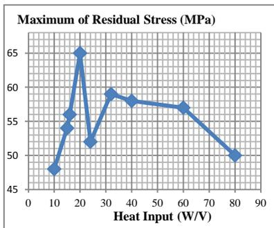
**Fig. 7.** Effect of W/V ratio on Residual Stresses of the as welded A356-SiC composites
