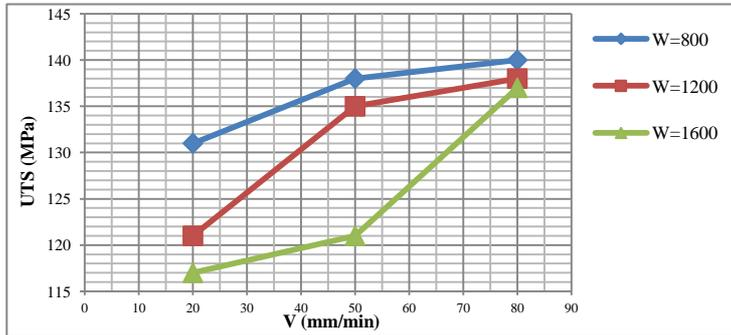
**Fig. 3.** Effect of V (transverse speed) and W (rotational rate) on Ultra Tensile Strength of the as welded A356-SiC composites
