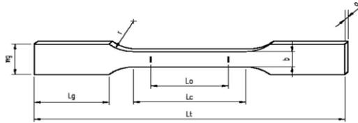
**Fig. 1.** Tensile test sample dimensions;  $a = 3\text{mm}$ ,  $w_g = 10\text{mm}$ ,  $L_g = 30\text{mm}$ ,  $L_c = 32\text{mm}$ ,  $r = 6\text{mm}$ ,  $b = 6\text{mm}$ ,  $L_o = 25\text{mm}$  and  $L_t = 100\text{mm}$ .
