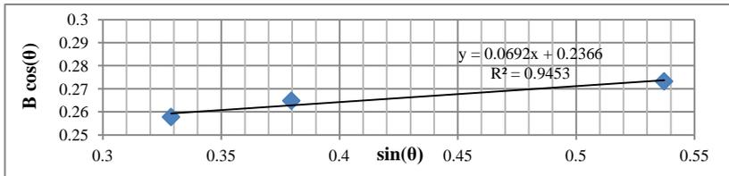
**Fig. 2.** An example of calculating  $\varepsilon$  from the XRD results via Williamson-Hall equation
