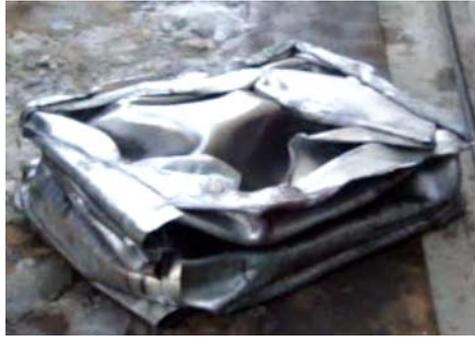
**Fig. 5.** Final compacted aluminium-coil waste
