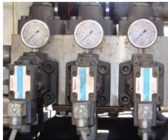
**Fig. 3.** manometers for measuring the force of cylinders
