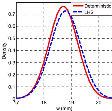
**Fig. 6.** Comparison of Gaussian probability density functions of calculated deflections from the ensemble provided by all 20 beams.
