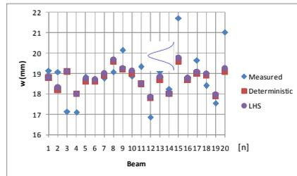
**Fig. 7.** Comparison of measured and calculated deflections (the circles show averages from 100 realizations obtained for individual beams).
