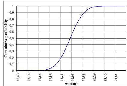
**Fig. 5.** Example of the Gaussian distribution function of deflection for the selected beam.
