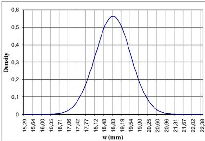
**Fig. 4.** Example of the Gaussian probability density function of deflection for the selected beam.
