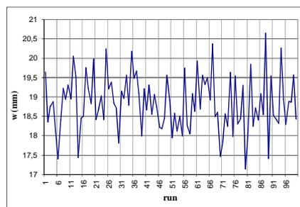
Fig. 3. Resulting maximal deflections for a single beam from one hundred realizations.
