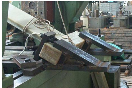
Fig. 4. Attachment of the GRP T-piece to the machine using the specially designed and manufactured gear
