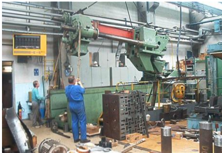
Fig. 3. SCHENCK PBVH machine being equipped with load multiplier
