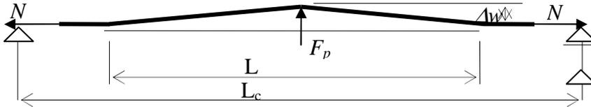
**Fig. 2.1** Principle of measurement of forces in a cable
