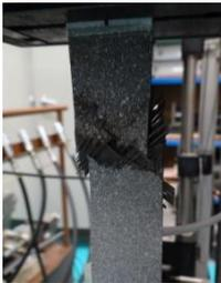
**Fig. 3.** Detail of tensile fracture of the specimen.
