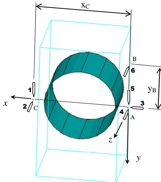
**Fig. 1.** Arrangement of six displacement transducers for the vibration measurement.
