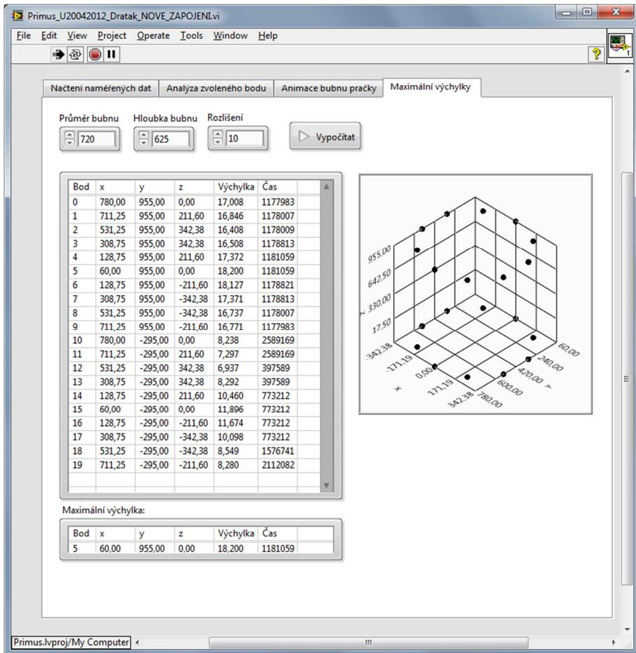
Fig. 3. Evaluation of the maximal deflection for the weights regime.
