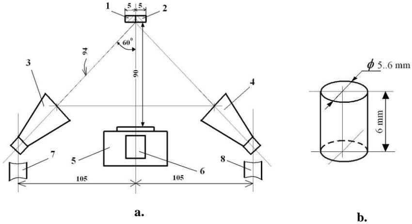
**Fig. 2.** Experimental set-up (a) and dimensions (in mm) for the tested specimen (b) [16, 17].
