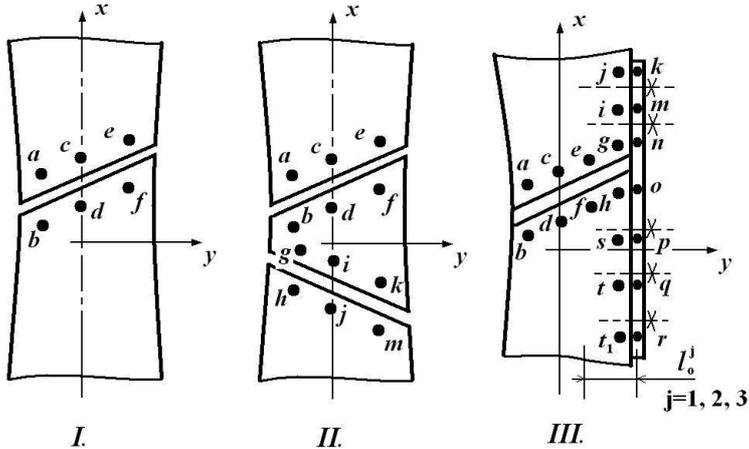
**Fig. 3.** The selection modality of the significant/interesting points on the tested bones: *I*, a simply unstable fracture; *II*, A multiple fractured bone; *III*, The case of the plate-fixators [2, 3].
