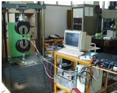
**Fig. 2.** Measurement of inductance variation of a specimen with a tensile load.
