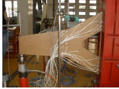
**Fig. 10.** View of deep beam failure
