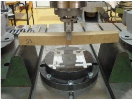
**Fig. 2.** Medium density fibreboard specimen subjected to flexural strength testing
