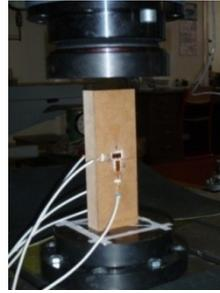
**Fig. 7.** Specimen in testing machine during compressive strength testing parallel to fibres
