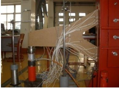
**Fig. 9.** Model with resistance strain gauges and inductive gauges, ready for testing
