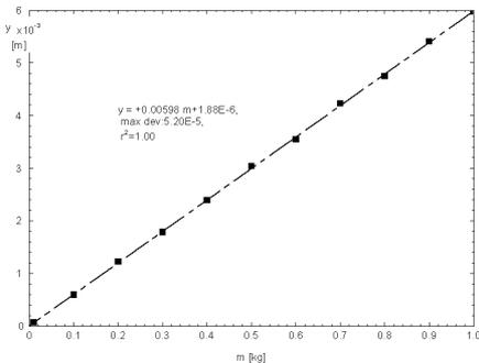
**Fig. 7.** Cantilever deflection ( $y$  – deflection,  $m$  – load)
