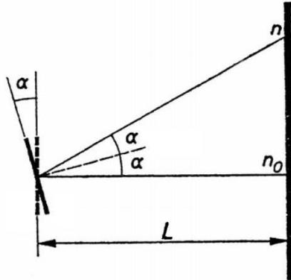
Fig. 3. Angle measuring by a mirror
