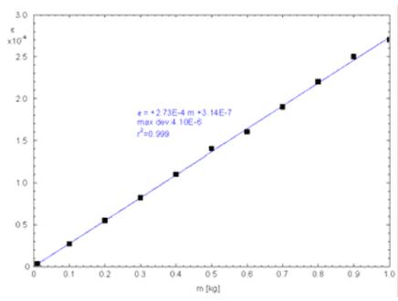
**Fig. 8.** Cantilever strain ( $\epsilon$  – strain,  $m$  – load)
