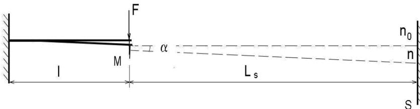
Fig. 4. Using a mirror to measure deflection of the cantilever ( $M$  – mirror,  $S$  – scale,  $F$  – force,  $l$ ,  $L_s$  – length,  $\alpha$  – angle,  $n$ ,  $n_0$  – units on the scale)
