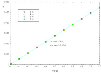
**Fig. 10.** Slope computed by means of a mirror ( $\alpha$  – angle,  $m$  – load)
