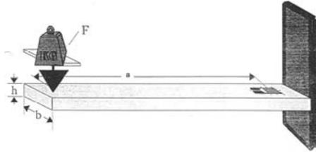
**Fig. 2.** Beam cantilever with strain gauge
