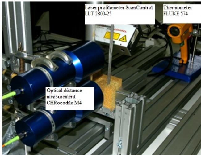
**Fig. 2.** Arrangement of the experiment.
