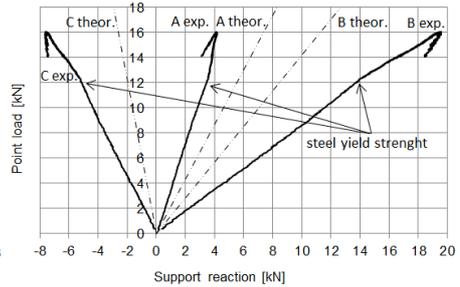
**Fig. 7.** Load-reaction diagram
