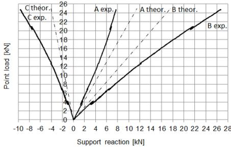
**Fig. 6.** Load-reaction diagram
