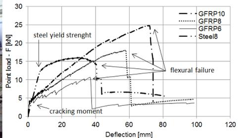
**Fig. 3.** Load-deflection diagram
