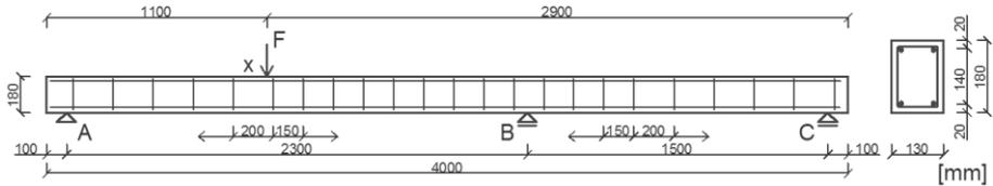
**Fig. 1.** Continuous beam reinforcement layout
