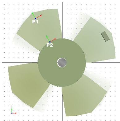
**Fig. 2. Model of cooling fan created in MSC.Adams/View**
