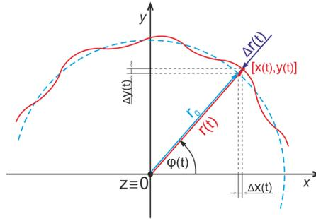
**Fig. 1. Estimation of vibration amplitudes of a rotating object**
