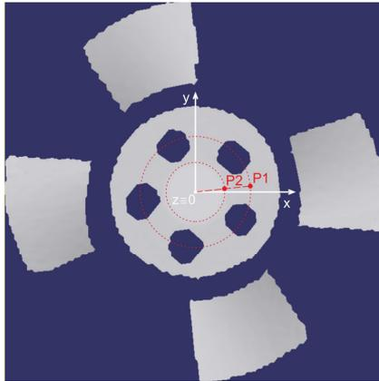
**Fig. 8.** Reconstructed spatial contour of cooling fan with measurement points
