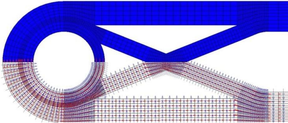
**Fig.7.** Directions of orthotropy in finite element model of double-crossed wrapping conception.
