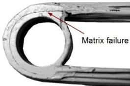
**Fig.3.** Simple conception matrix failure.
