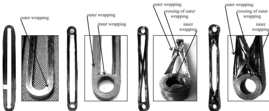
**Fig. 1.** Original tension sample (left) and tension/compression (simple, crossed and double-crossed) conceptions [4].
