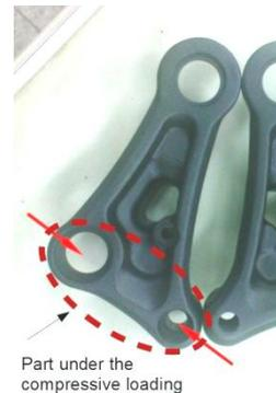
Fig.14. Linkage part under compression
