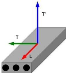
**Fig.8.** Directions of orthotropy in general unidirectional composite.
