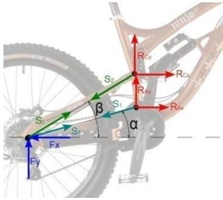
**Fig.15.** Joint method scheme.
