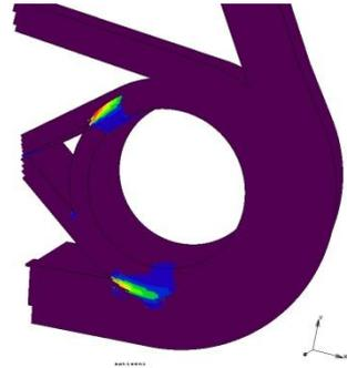
**Fig.17.** Critical locations according to linkage model (adjusted LaRC04, mode 2).
