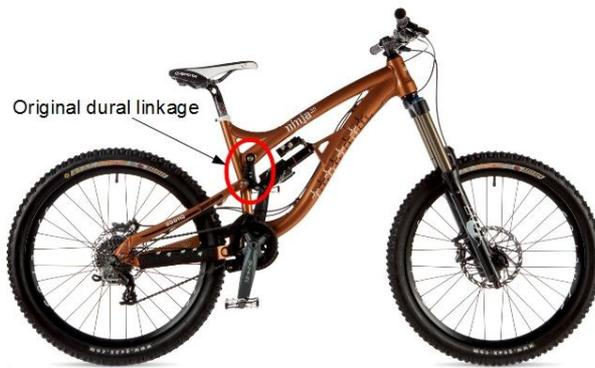
Fig.13. Original Dural linkage on bicycle with 180mm rear travel.
