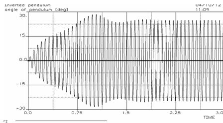
**Fig. 5.** Time history of pendulum angle  $\varphi$  [deg], excitation frequency  $f = 17$  Hz.
