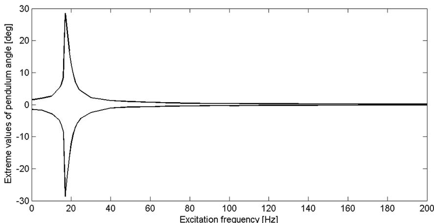
**Fig. 3.** Extreme values of time histories of pendulum angle  $\varphi$  in dependence on excitation frequencies.
