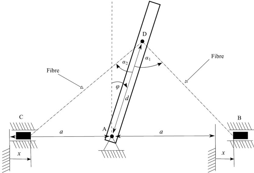
**Fig. 1.** Inverted pendulum actuated by the fibres.
