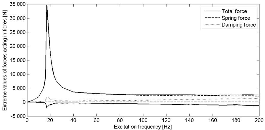
**Fig. 4.** Extreme values of time histories of forces acting in fibres in dependence on excitation frequencies.
