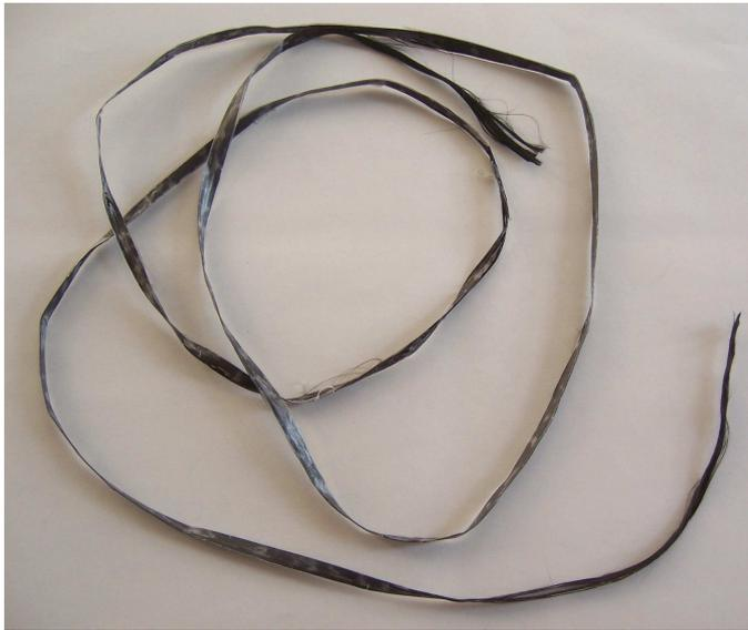
Fig. 2. “Light” fibre made of thin carbon fibres.
