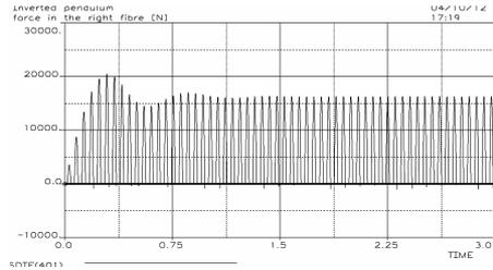
**Fig. 8.** Time history of force [N] acting in fibre 1, excitation frequency  $f = 19.4$  Hz.
