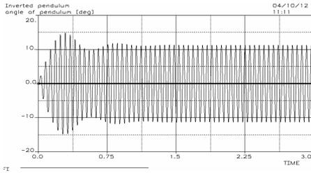
**Fig. 7.** Time history of pendulum angle  $\varphi$  [deg], excitation frequency  $f = 19.4$  Hz.
