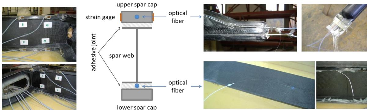
**Fig. 3** Sensors placement scheme with details of ingress/egress points of optical fibers and strain gages cabling.
