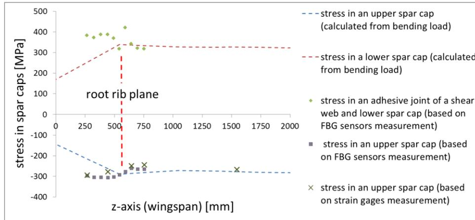
**Fig. 6** Stress distribution in the spar caps over the wingspan (operational load level) .
