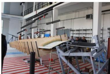
**Fig. 4** Wing in the fixture.
