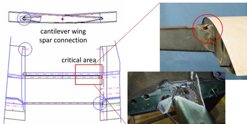
**Fig. 1** Principal of demountable cantilever wing, with details of critical area of a cantilever spar.
