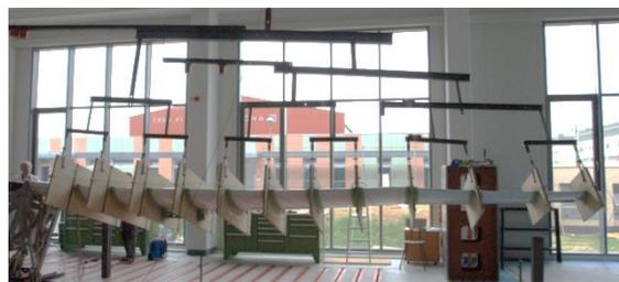
**Fig. 5** Configuration for bending load test.
