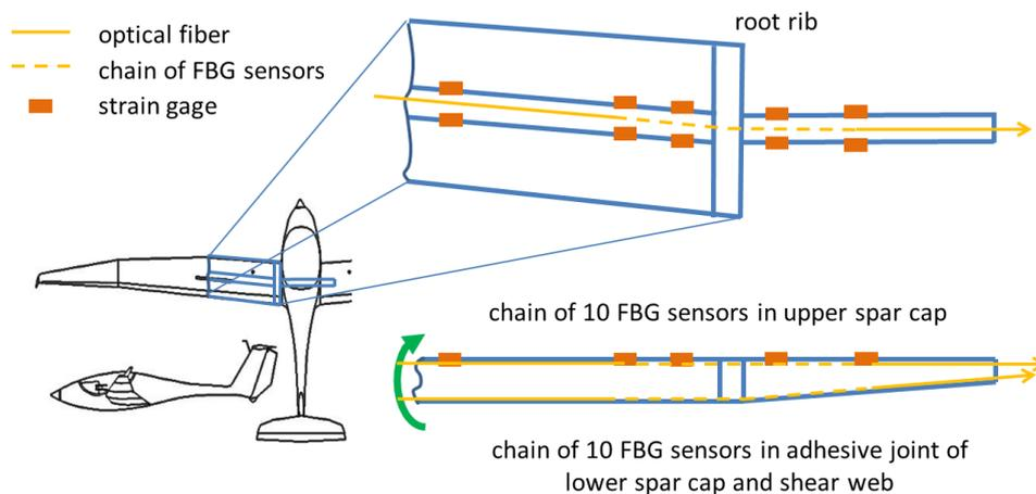
**Fig. 2** Location of the FBG sensors and strain gages on the wing spar.
