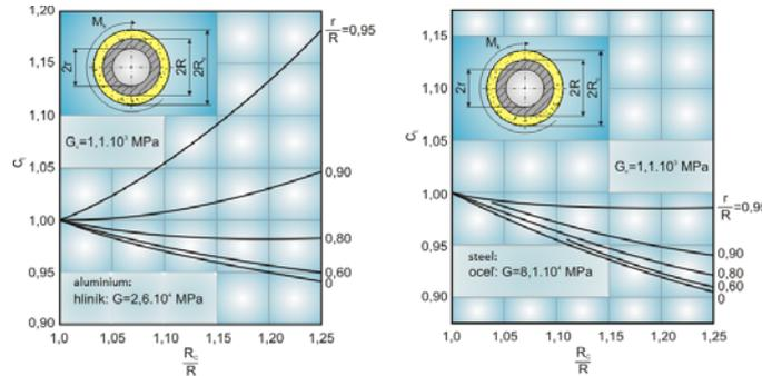
Fig. 3 Correction coefficients during torsional loads on shafts
