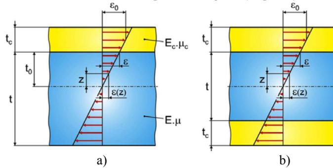
Fig. 2 Coating of an object under bending loads
