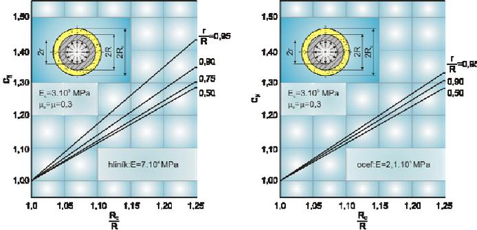
Fig. 4 Correction coefficients in pressure vessel
