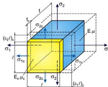
Fig. 1 Stress state and deformation in the structure and its coating in the event of plane stress state
