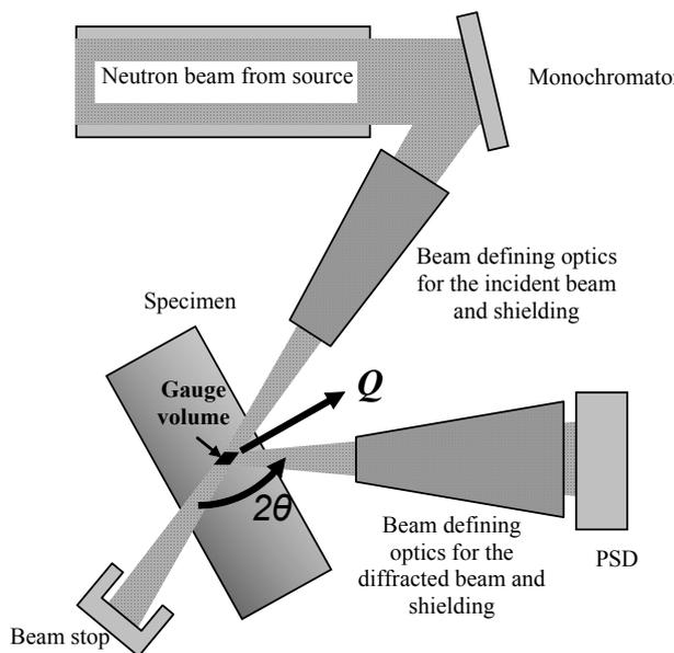
Fig. 3. Schematic illustration of a reactor source based diffractometer for strain measurement in parallel diffraction geometry.
