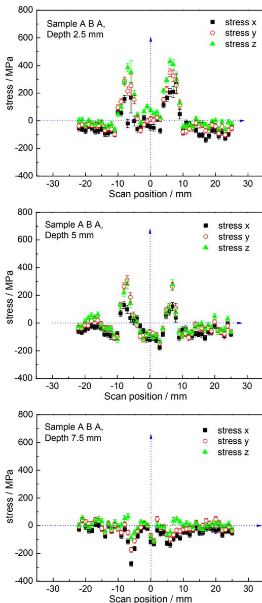
Fig. 5. Residual stress scans performed at different depths in the material for the sample with the weld on one side.
