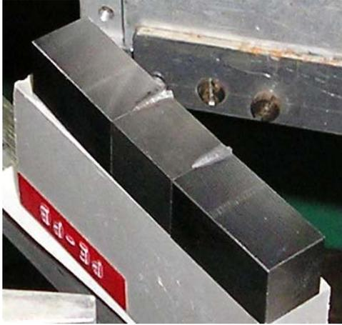
Fig. 1. Photo of one of the specimens with the weld on one side.
