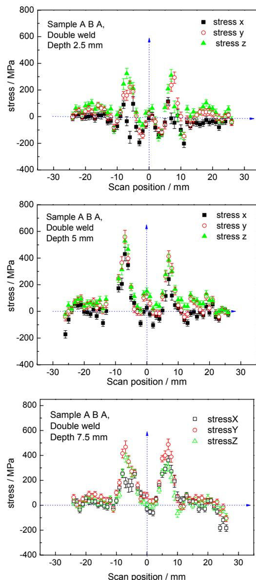
Fig. 6. Residual stress scans performed at different depths in the material for the sample with the weld on both sides.
