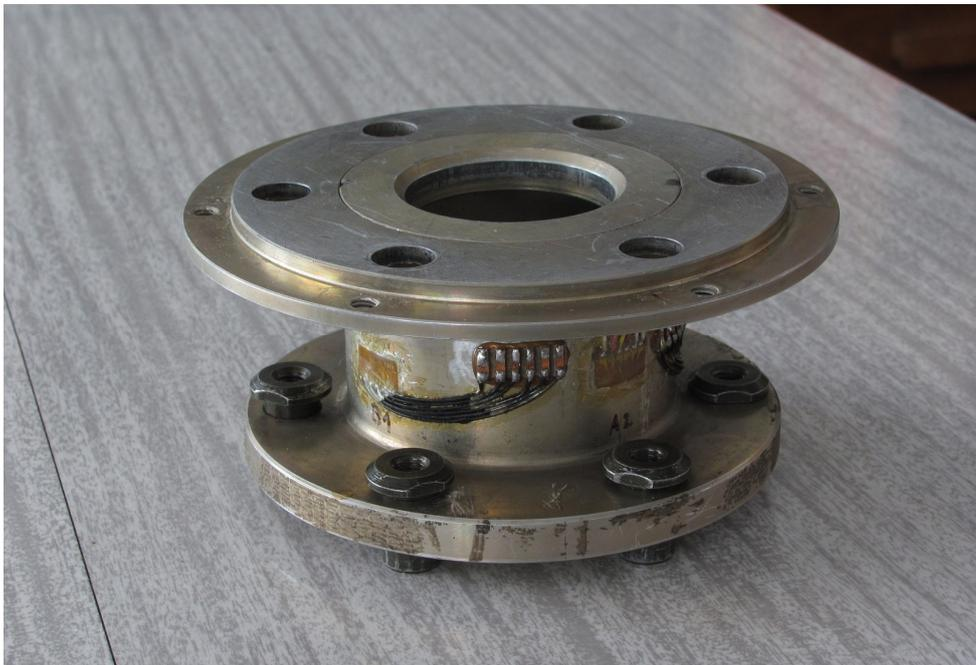
**Fig. 2.** Special shaft element equipped with strain gauges.
