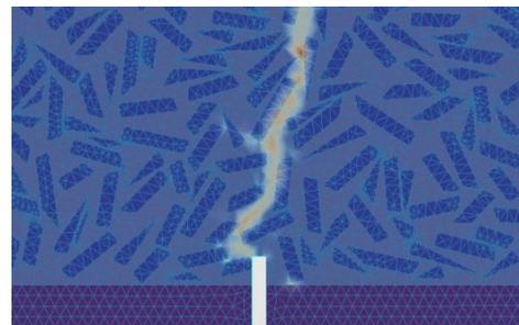
b) splitting test (fine crushed brick particles)
