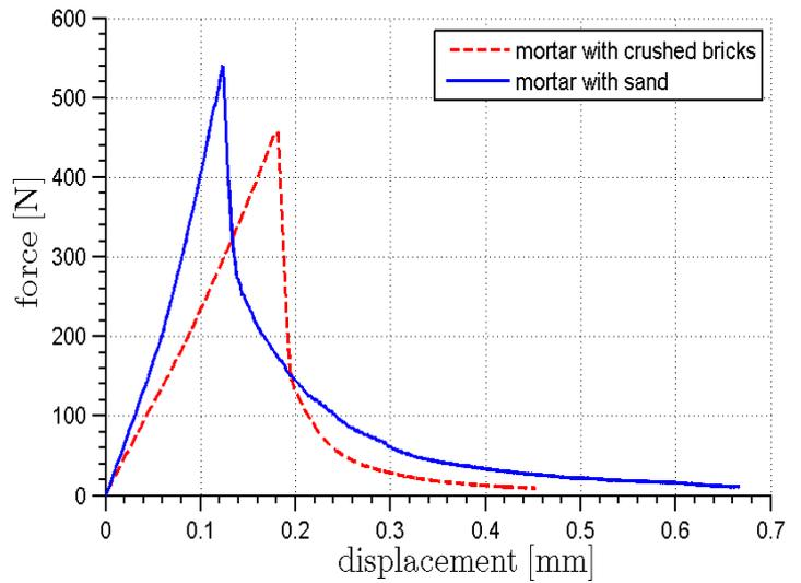
Fig. 3: Typical load-displacement diagrams for mortars containing aggregates in volumetric fraction equal to 0.48 obtained from measurements during three-point bending test
