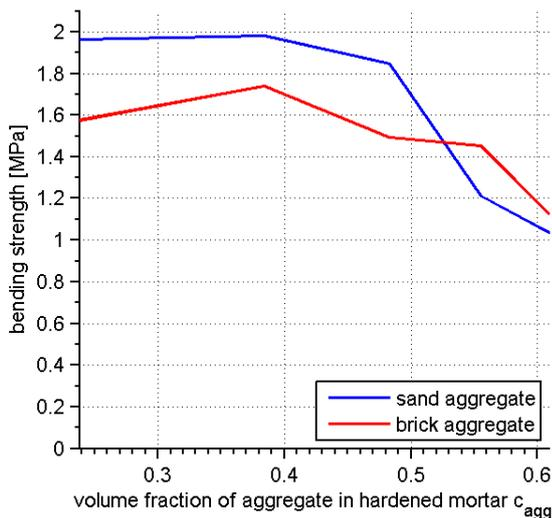
Fig. 4: Dependence of mortar bending strength on volume fraction of aggregates
