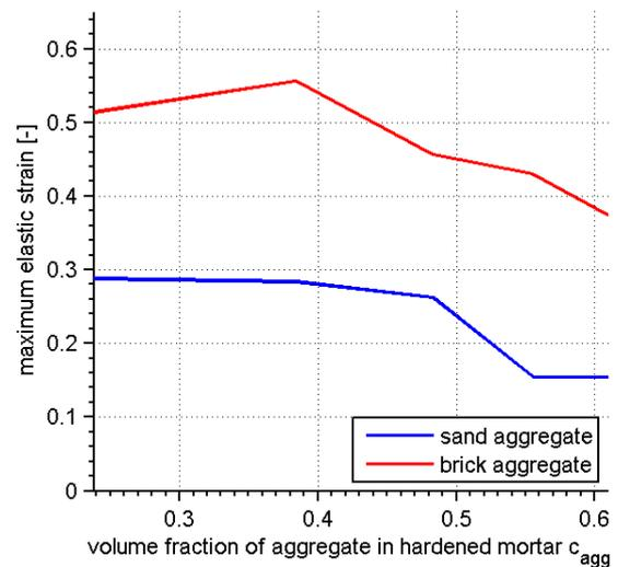
Fig. 5: Dependence of mortar limit elastic strain on volume fraction of aggregates
