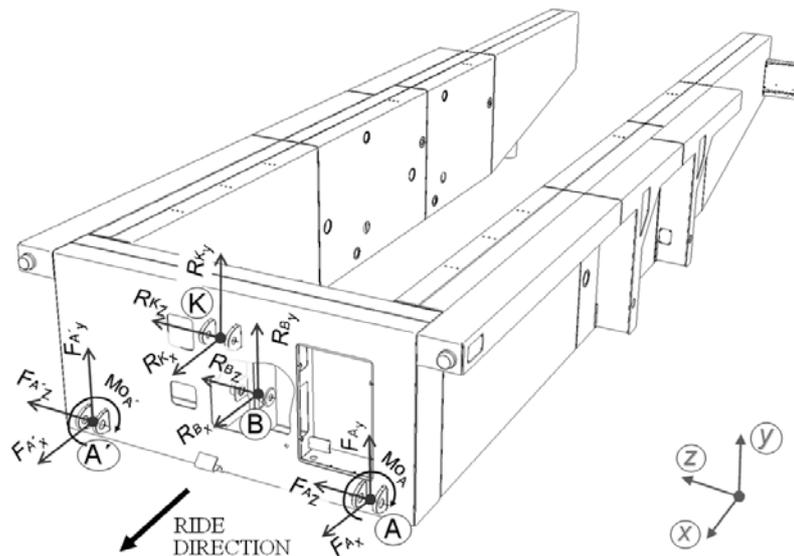
Fig. 3 – Applied reactions on part of trailer frame
