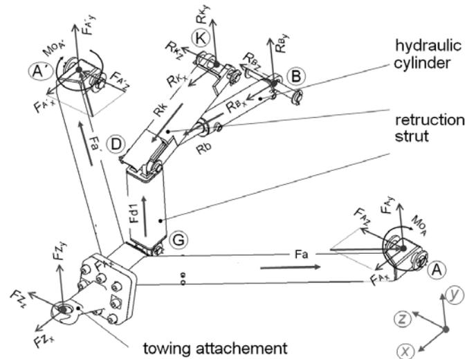
Fig. 2 – Application forces and reactions on trailer hitch
