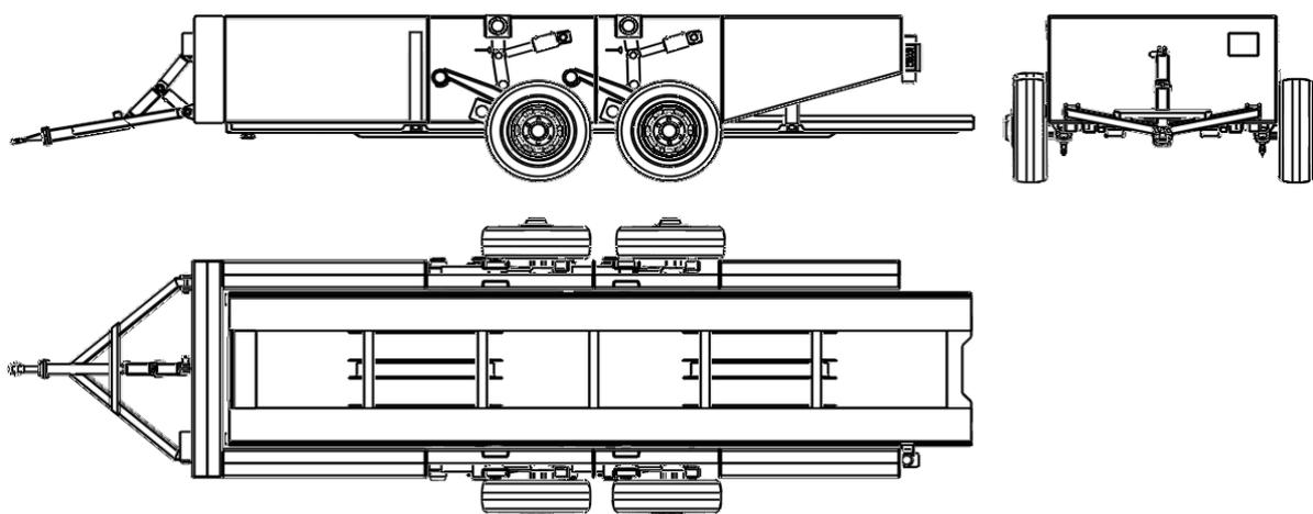
Fig. 1 – Developed agricultural self-loading trailer
