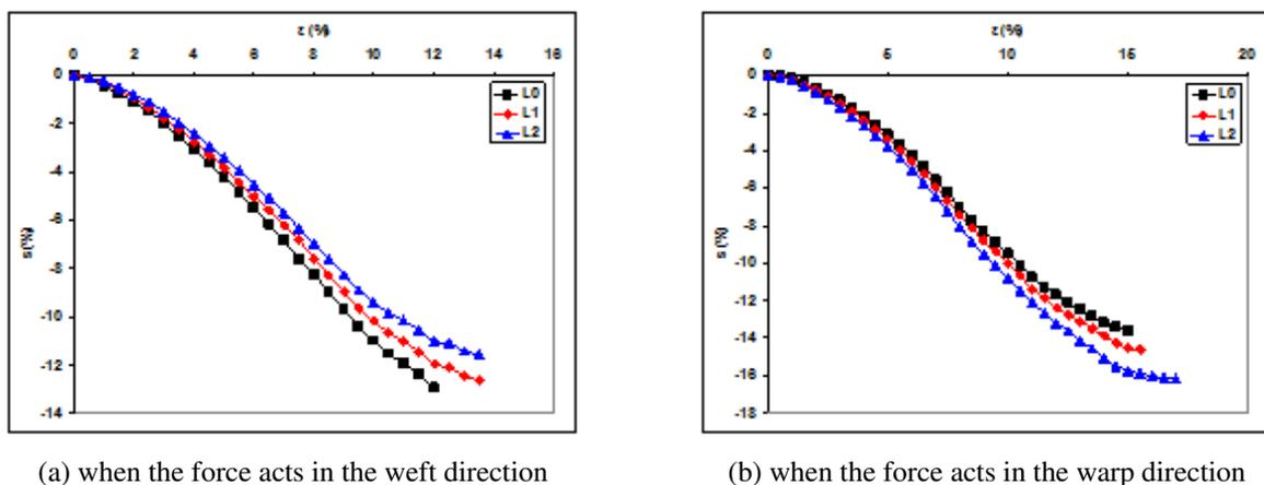
Fig. 2: Diagram of relative contraction of fabric  $s$  (%).
