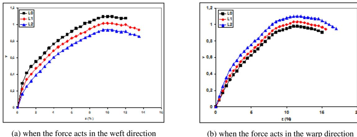
Fig. 3: Poisson's ratio  $\nu$  of the fabric.
