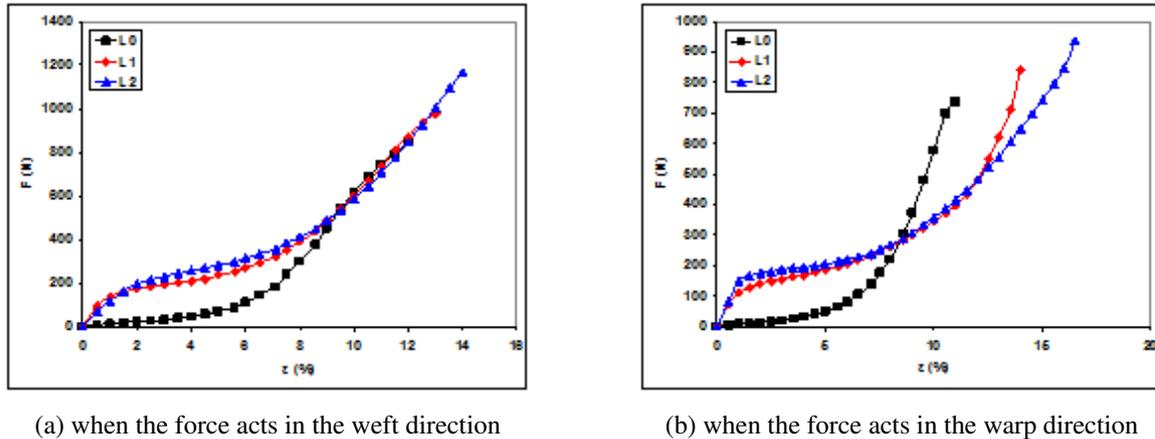
Fig. 1: Tensile force-elongation diagram ( $F-\varepsilon$ ) till rupture.
