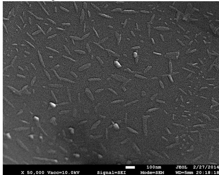
Fig.1: Distribution of carbon nanotubes.
