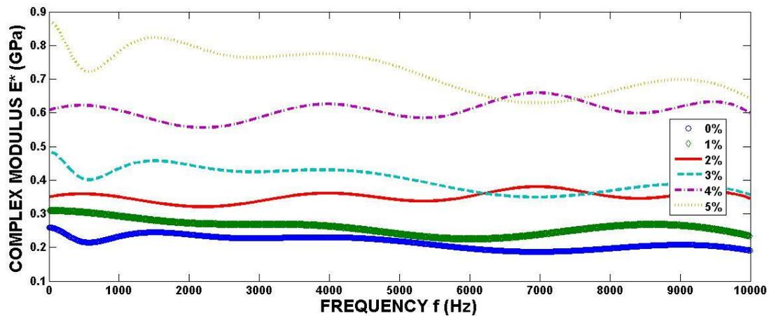
Fig.8. Complex modulus of tested specimens.
