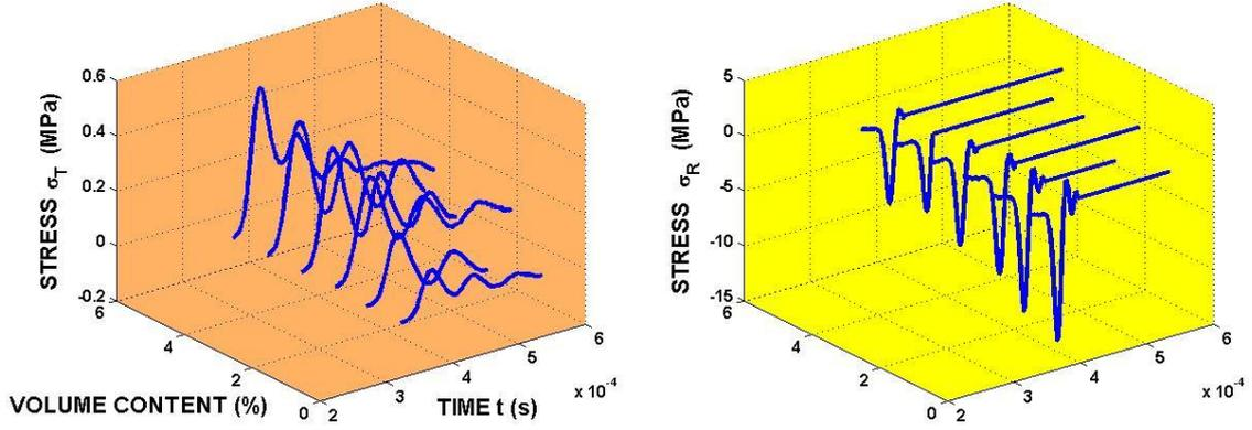
Fig.5: Experimentally recorded transmitted,  $\sigma_T$ , and reflected,  $\sigma_R$ , stress pulses.
