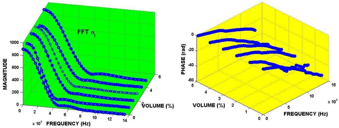
Fig.6: Spectral characteristics of the incident stress pulses.
