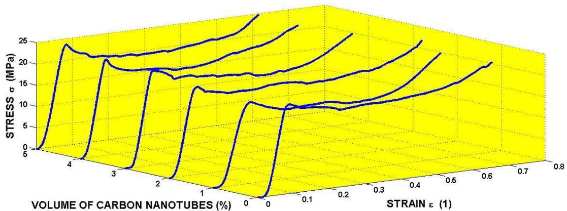
Fig.2: Stress strain curves at static compression.
