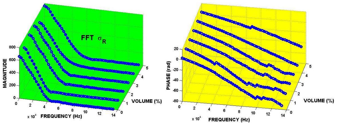
Fig.8: Spectral characteristics of the reflected stress pulses.
