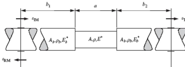
Fig. 3: Schematic of the central part of SHPB setup showing test specimen placed between two pressure bars.
