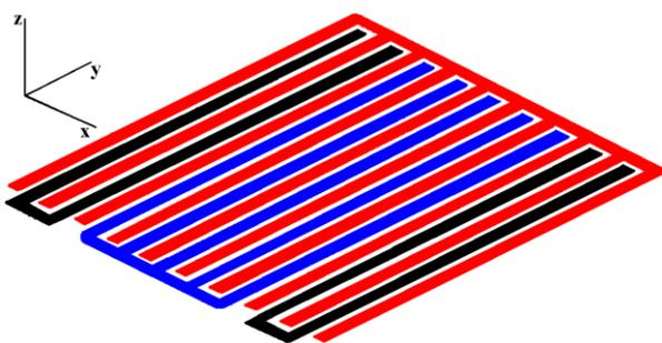
a) An arrangement of FEF sensor coplanar electrodes;
