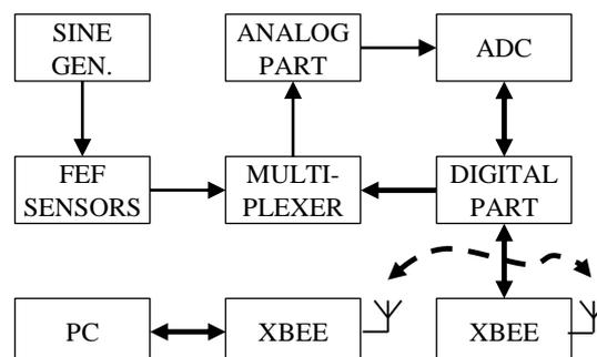
Fig. 4: Schematic diagram of main components of the monitoring system;
