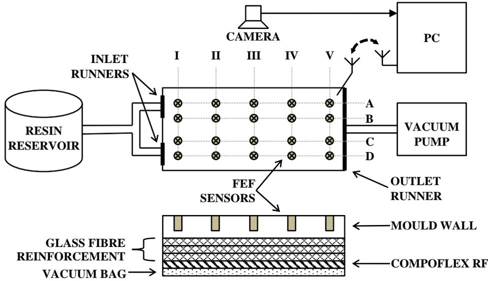
Fig. 6: Schematic setup of the experimental demonstration;
