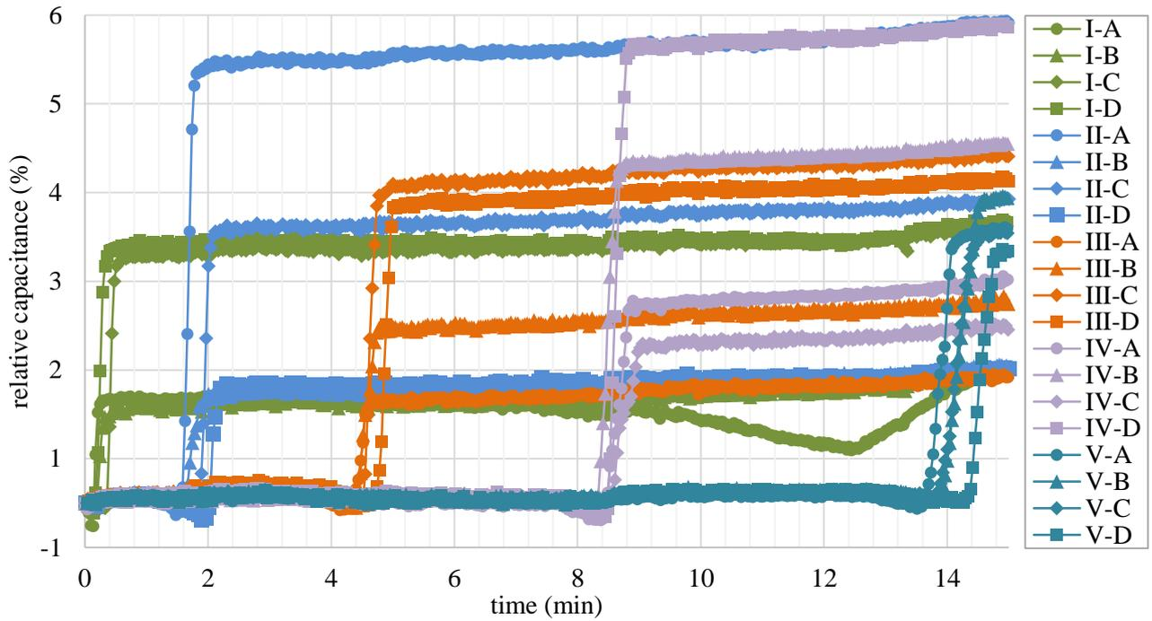
Fig. 7: The sensor relative capacitance changes during filling process;
