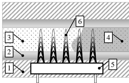
Fig. 3: Side view of FEF sensor installed in the mould wall. (1-mould, 2-gelcoat, 3-fabric, 4-fabric&resin, 5-sensor, 6-FEF);
