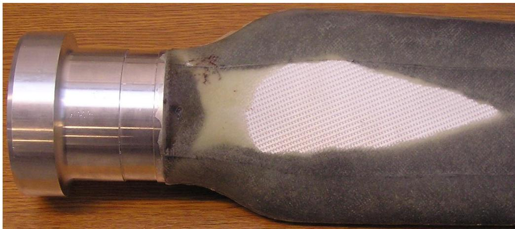
Fig. 1: An example of a typical dry spot;
