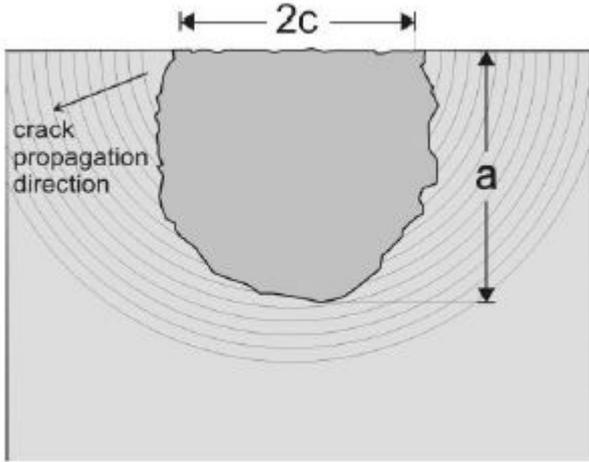
Fig. 3: Schematic Illustration of Pit Geometry
