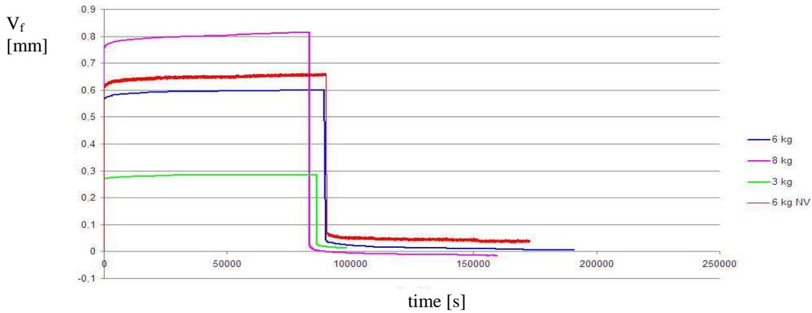
Fig. 2 Vertical displacement vs time in bending of sandwich beam
