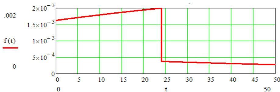
**Fig. 1** Strain vs time in compression of sandwich core
