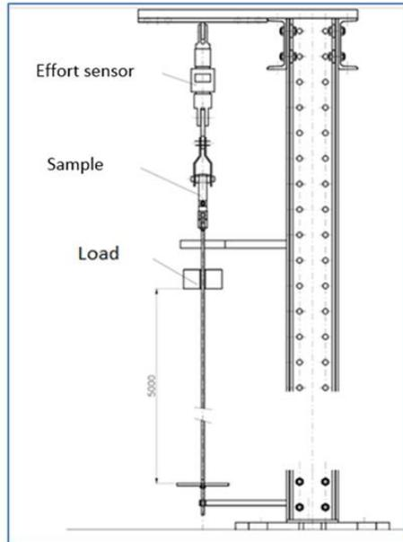
Fig. 3: Drop test set up
