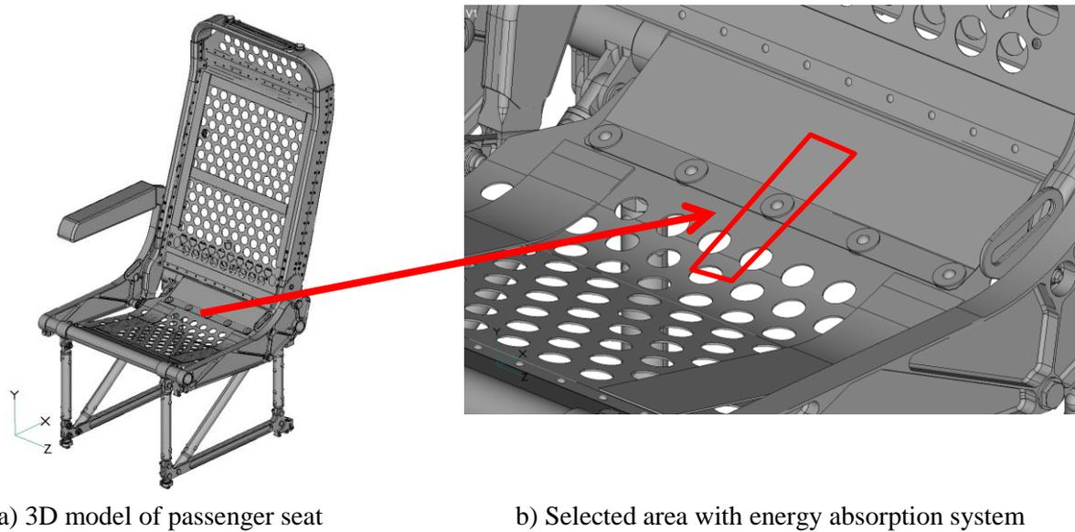
Fig. 1: Passenger seat with application of energy absorption system
