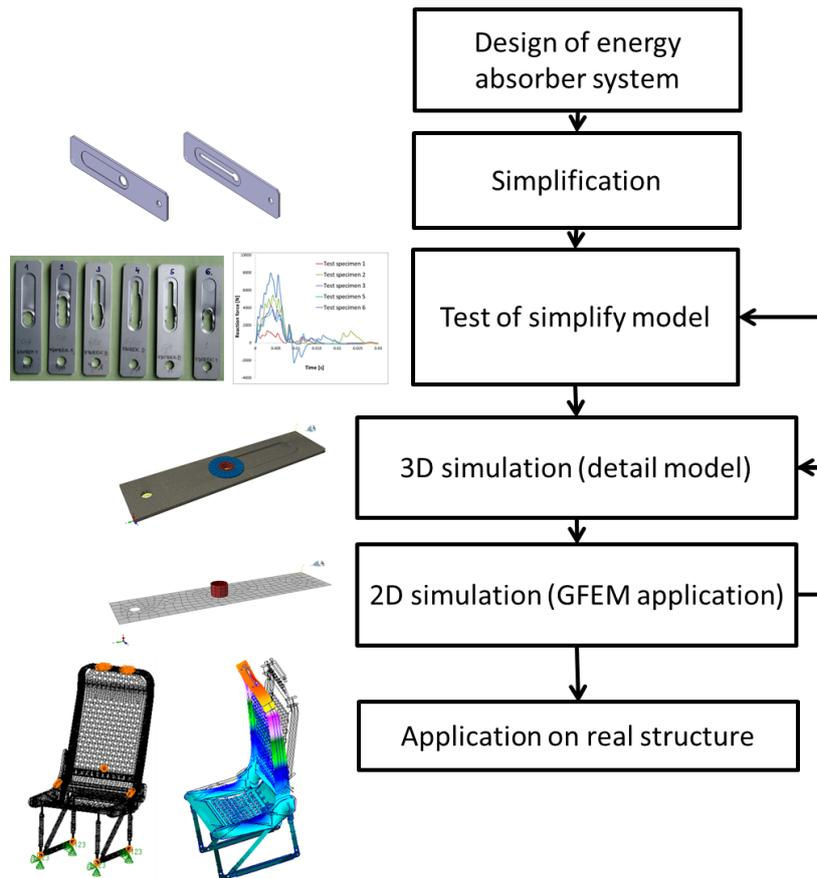
Fig. 8: Shema of energy absorption system design and optimization
