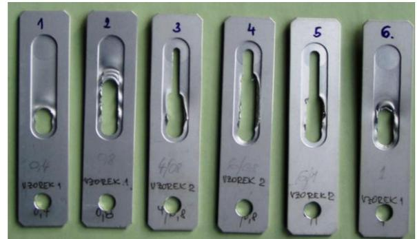
b) Deformed shape of test specimen
