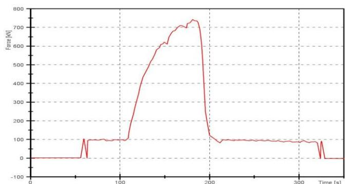
Fig. 5: Record of the forging force curve of the second raw product.
