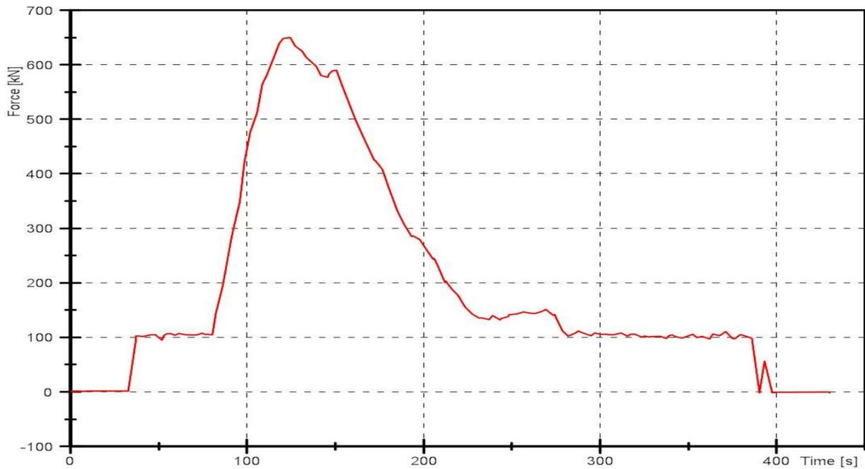
Fig. 3: Record of the forging force progress in time during the whole length of operation of the forging machine.
