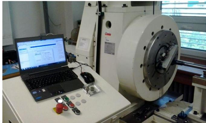
Fig. 2: Forging machine with the installed measurement system.
