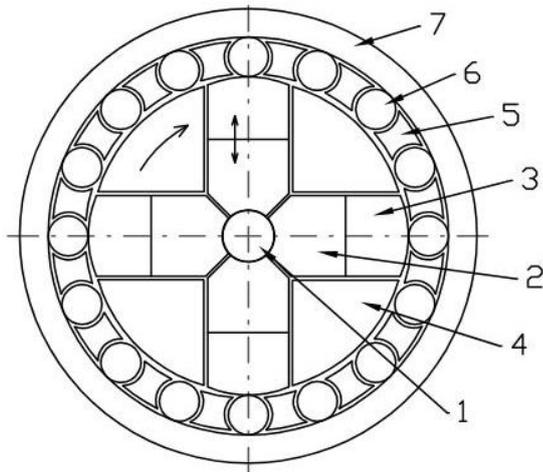
Fig. 1: Rotary swaging principle.
