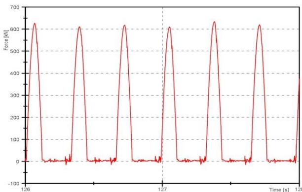
Fig. 4: Cut of the real forging force curve in time during forging (swaging).
