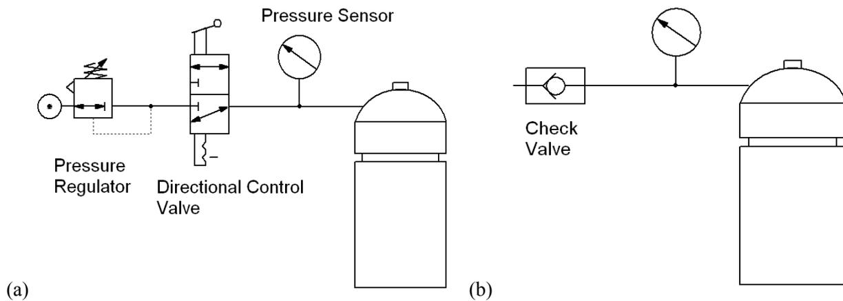
Fig. 3: (a) Setup of bottle sealing test, (b) Setup of check valve connection.
