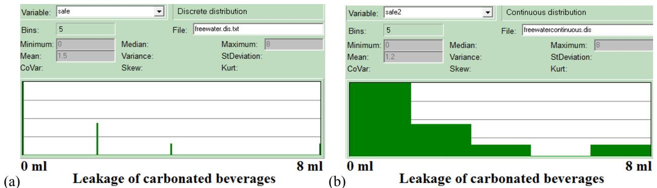
Fig. 6: Plastic bottle with a “sports cap” closure (statistical evaluation of the volumes of liquid leakage for carbonated beverages – (a) discrete histogram, (b) continuous histogram).
