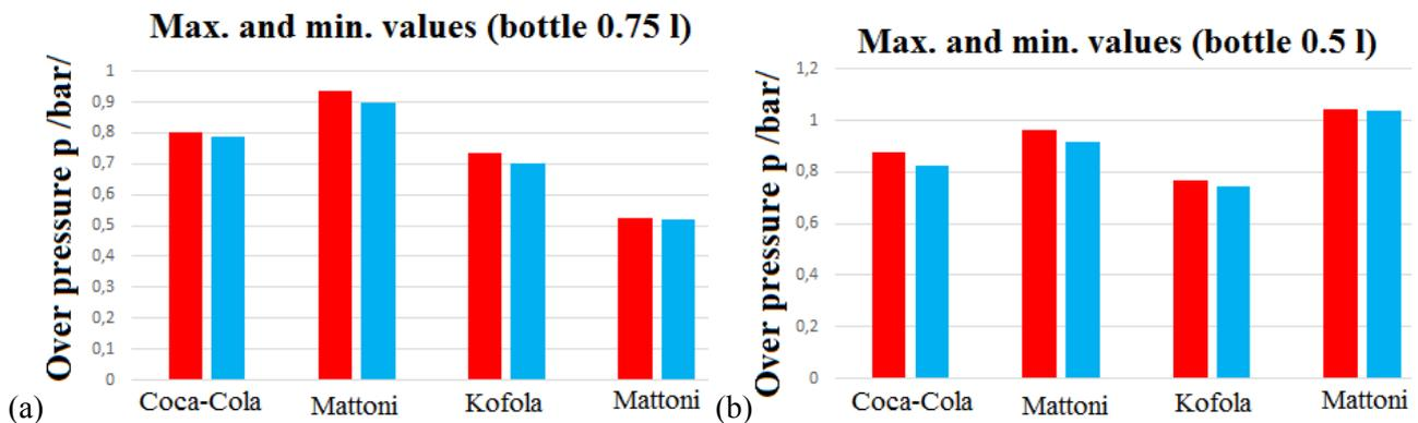
Fig 5: Plastic bottles with the “sports cap” closure (max. and min. overpressure when containing carbonated beverages).
