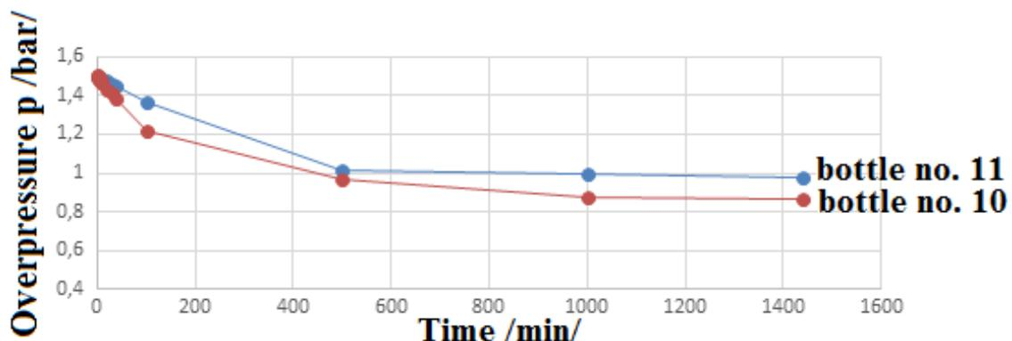
Fig 4: Graph of overpressure decrease (leakage from bottle) – results of 24-hour measurement.
