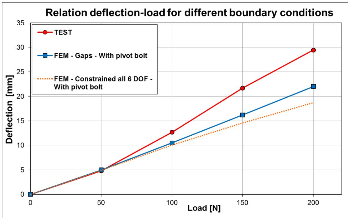
Fig. 10: Comparison of nacelle deflection for different boundary conditions
