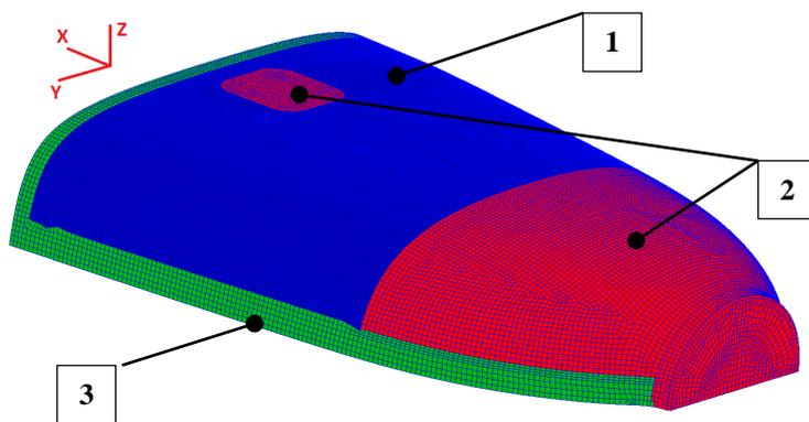
Fig. 3: Positions of monolithic laminate and sandwich composite
