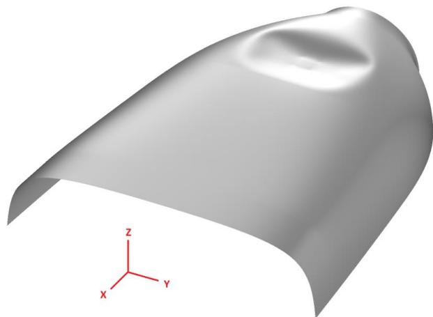
Fig. 8: Deformation shape of nacelle with gap elements on free edges
