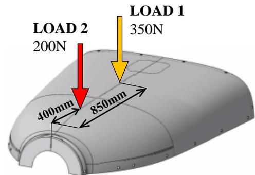
Fig. 4: Positions of loading
