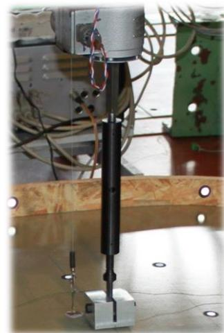
Fig. 2: Loading support foot
