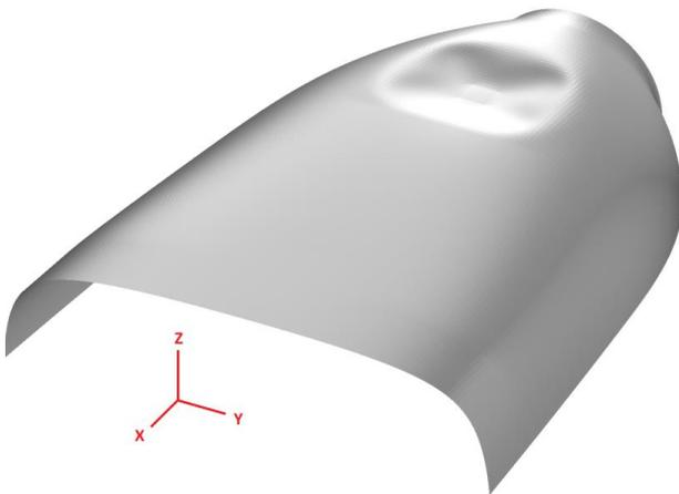
Fig. 7: Nacelle with constrained all 6 degrees of freedom on free edges
