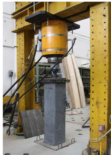
Fig. 4: Tested column in the loading press.
