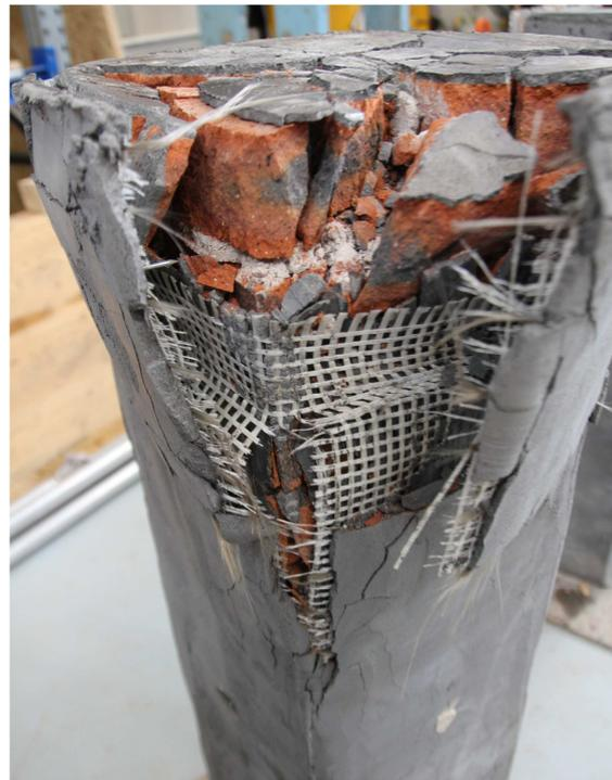
Fig. 6: Detail of collapsed strengthening layer and column after performed test.
