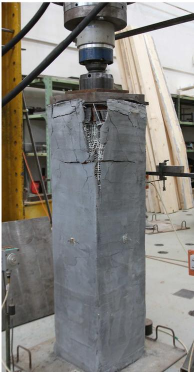
Fig. 5: Tested strengthened column.
