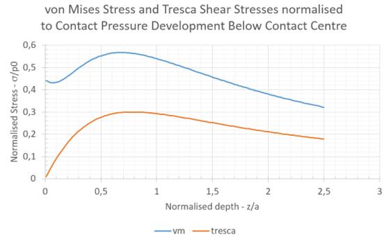
Fig. 7: Normalised development of sub-surface stresses Tresca and von Mises. Analytical solution, valid only in elastic domain.
