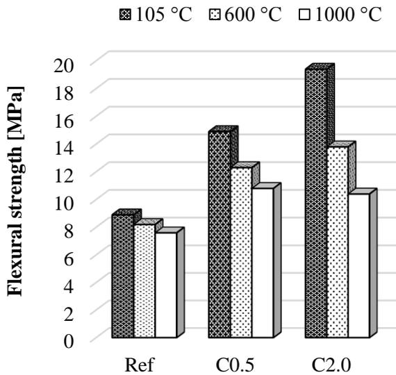
Fig. 1: Values of flexural strength.
