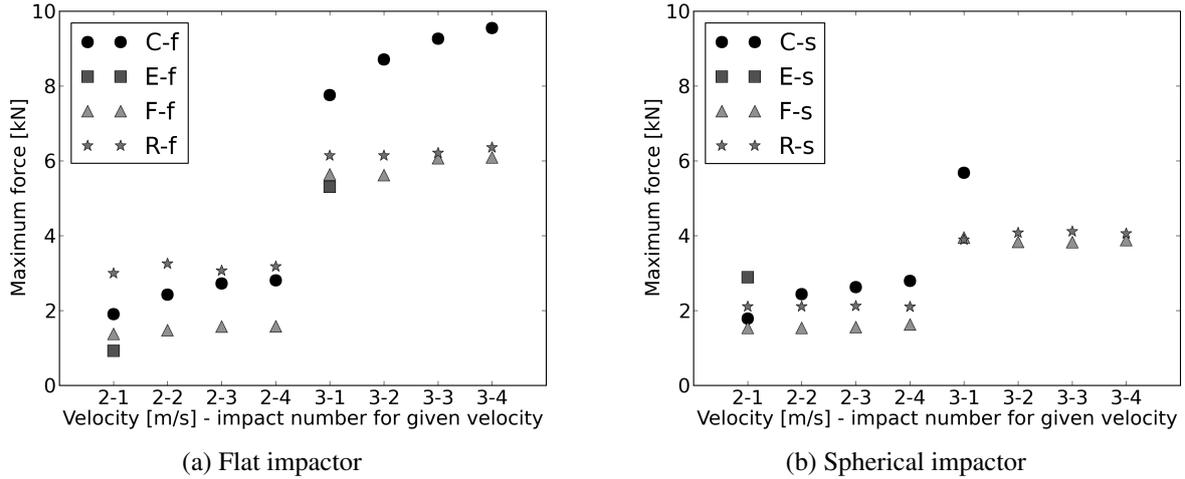
Fig. 12: Maximum force (MF) dependence on impact repetition.
