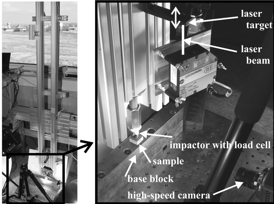
Fig. 1: Drop test.
