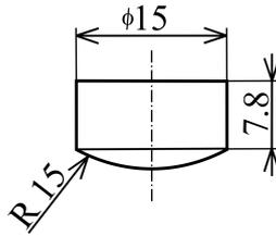
Fig. 2: Geometry of spherical impactor [mm].
