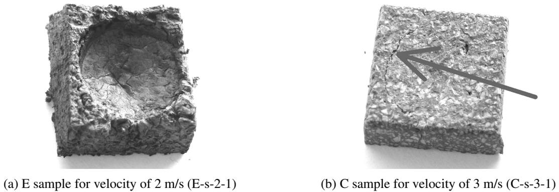
Fig. 13: Samples after test using spherical impactor.
