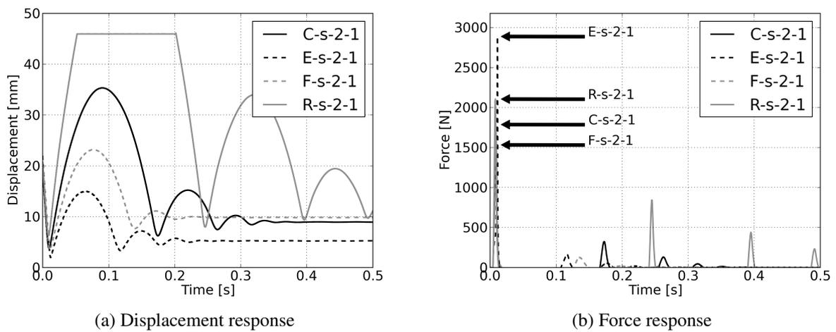
Fig. 5: Responses on impacts of spherical impactor for velocity of 2 m/s.
