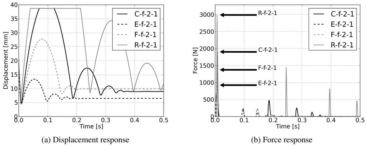
Fig. 3: Responses on impacts of flat impactor for velocity of 2 m/s.
