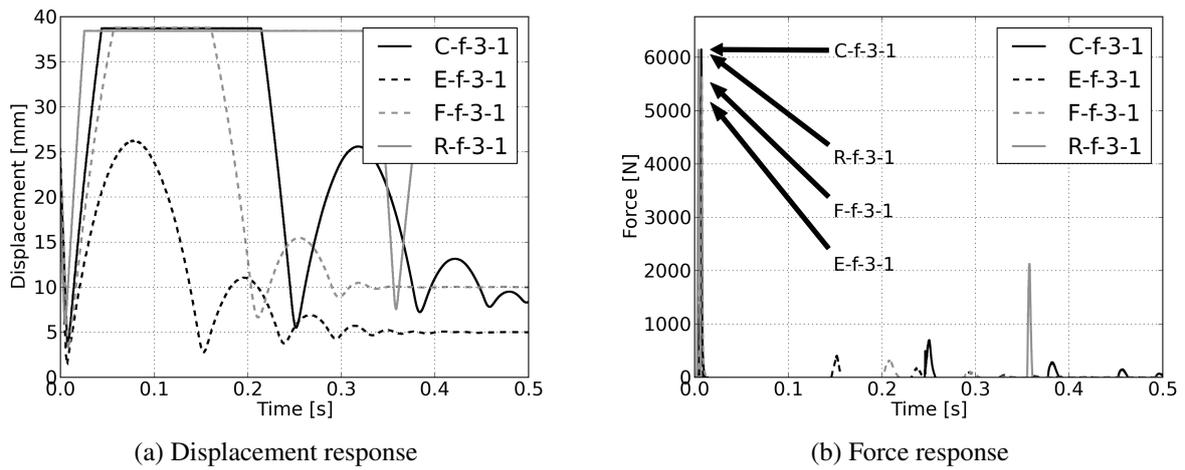
Fig. 4: Responses on impacts of flat impactor for velocity of 3 m/s.
