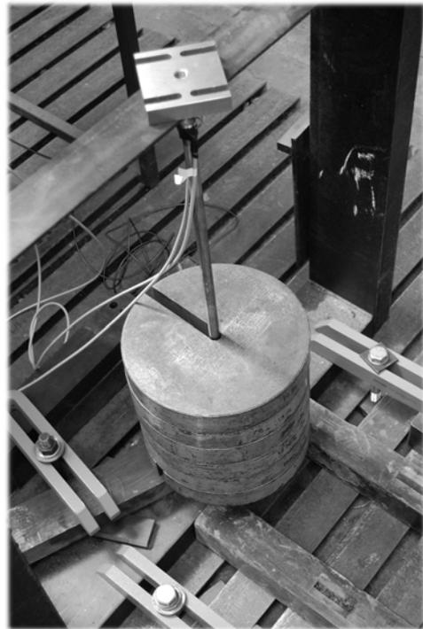
Fig. 8: The test stand for force gauge – loaded by weights
