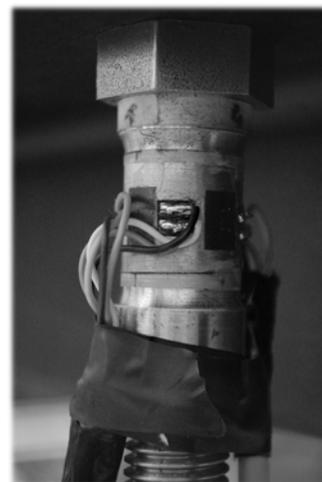
Fig. 6: Force gauge with semiconductor strain gauges and wires
