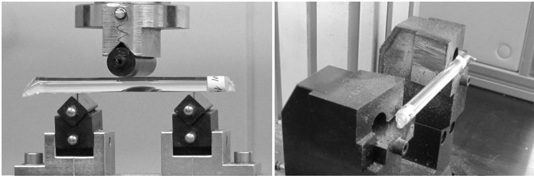
Fig. 1: Left – 3-point bend test; Right – Charpy test
