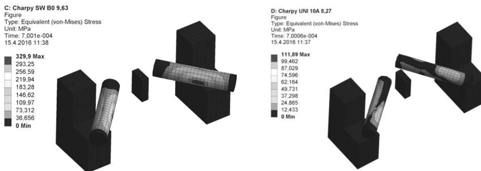
Fig. 6 and 7: Stress distribution during Charpy test for Type 1 and Type 2 sample
