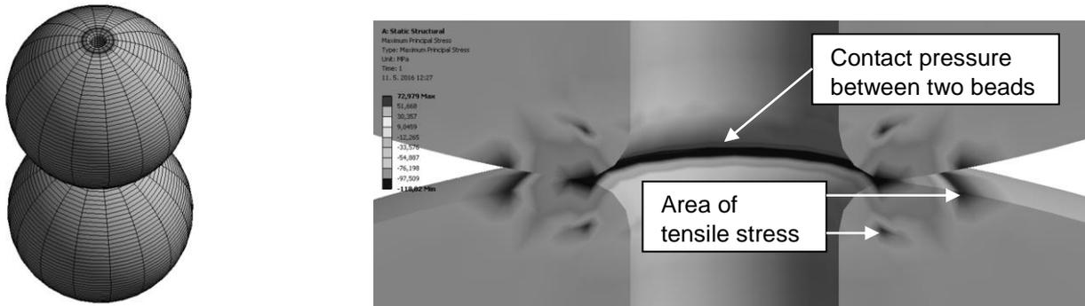
Fig. 8, 9: Model of beads pressed by the gravity force (left); a detail of contact pressure of two beads
