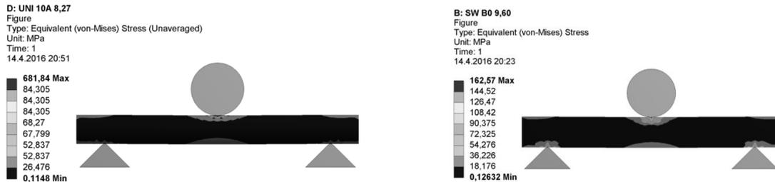
Fig. 3 and 4: Stress distribution in sample Type 1 and Type 2
