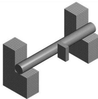
Fig. 5: Meshed geometry of Charpy test model
