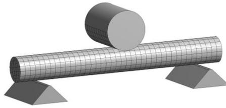
Fig. 2: Meshed geometry of 3-point bending test model
