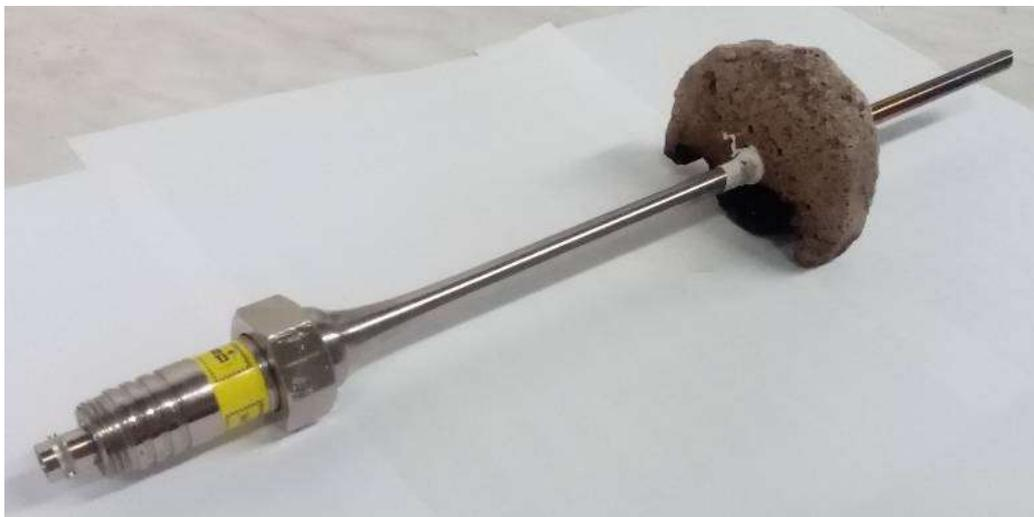
Fig. 2: The acoustic emission sensor on the waveguide
