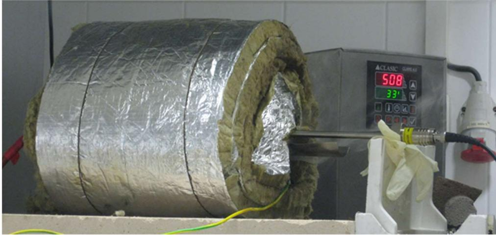
Fig. 1: The temperature loading of the specimen into a special oven and the position of the acoustic emission sensor on the waveguide
