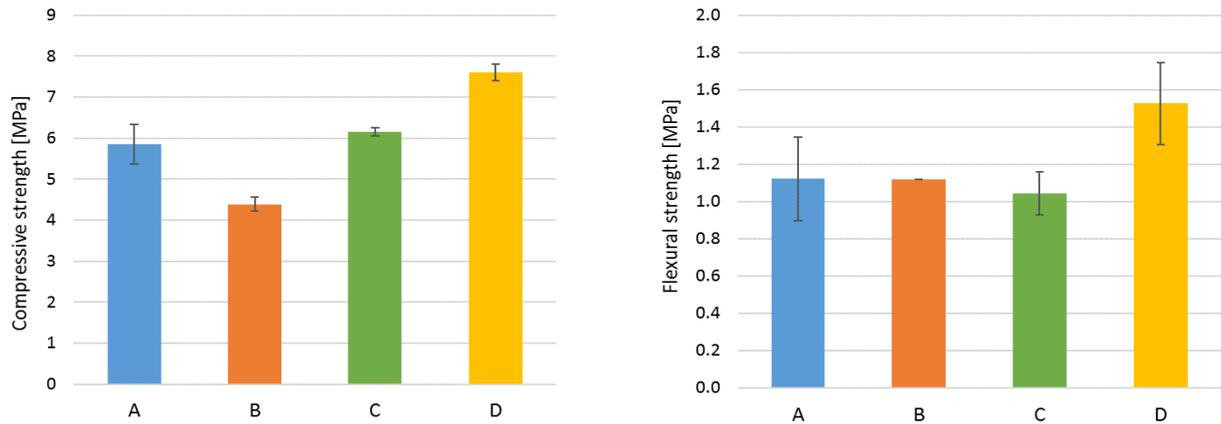
a) comparison of compressive strength (with standard deviation)
